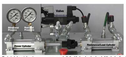
Illustrated above is how to measure pressure on both the blind-end and rod-end of the hydraulic cylinder.
