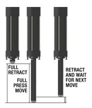
This illustration shows move comparison of a hydraulic press move on the left vs. electric press application on the right.
