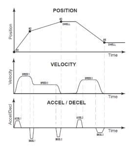
This chart shows different motion profile positions at different velocities with different accel/decel rates, all under full and precise control.
